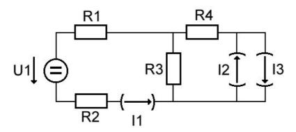
Werte:  $I_1 = I_2 = I_3 = 1A$ ,  $R_1 = R_2 = R_3 = 1\Omega$ ,  $U_1 = 1V$
