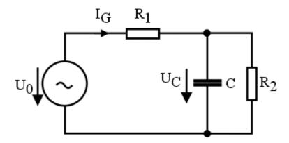
Werte:  $U_C = 5V$ , 50Hz,  $R_1 = 50\Omega$ ,  $R_2 = 100\Omega$ ,  $C = 16\mu F$
