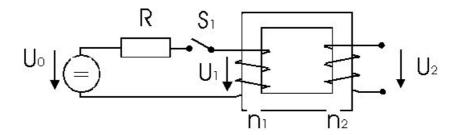
Werte:  $U_0 = 10V$ ,  $n_1 = 300$ ,  $n_2 = 150$ ,  $R_1 = 10 \Omega$ ,  $L_1 = 10 \text{mH}$
