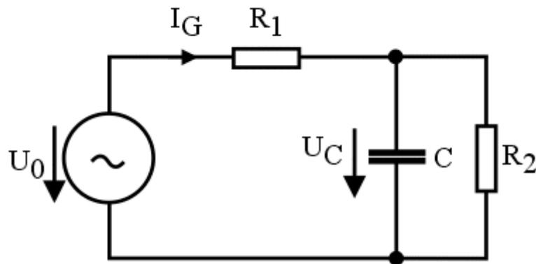
Werte:  $U_C = 5V$ ,  $50\text{Hz}$ ,  $R_1 = 50\Omega$ ,  $R_2 = 100\Omega$ ,  $C = 16\mu\text{F}$
