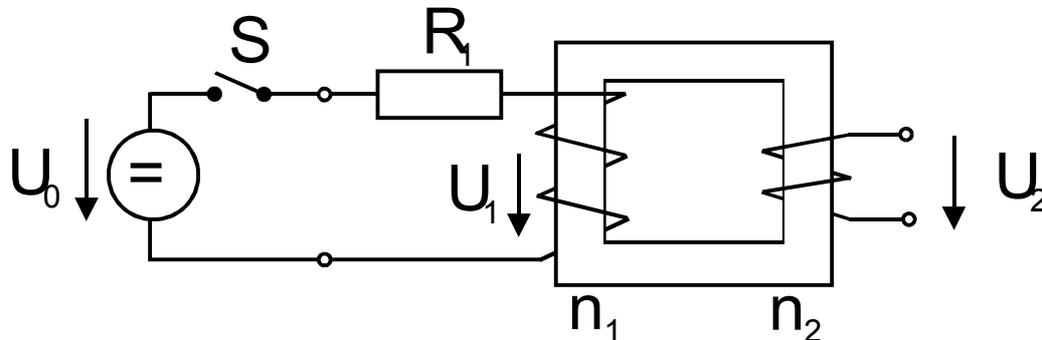
Werte:  $U_0 = 10\text{V}$ ,  $n_1 = 300$ ,  $n_2 = 150$ ,  $R_1 = 10\ \Omega$ ,  $L_1 = 10\text{mH}$
