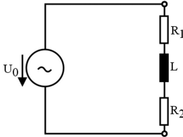
Werte:  $U = 230\text{V}$ ,  $f = 50\text{Hz}$ ,  $R_1 = 1\ \Omega$ ,  $R_2 = 50\ \Omega$ ,  $L = 64\text{mH}$
