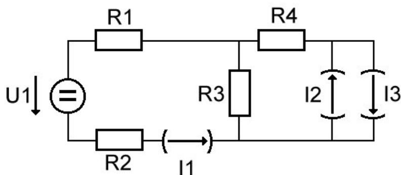
Werte:  $I_1 = I_2 = I_3 = 1\text{A}$ ,  $R_1 = R_2 = R_3 = 1\Omega$ ,  $U_1 = 1\text{V}$
