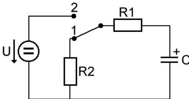
Werte:  $U = 10\text{V}$ ,  $R_1 = R_2 = 50\text{k}\Omega$ ,  $C = 100\mu\text{F}$
